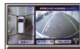
Display Example of OVM (images of OVM and rear view camera)
