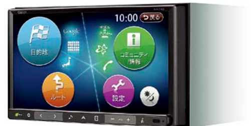
Smoonavi NX710 AV-Navi System with Wide 7-inch VGA Double-DIN Terrestrial Digital TV/DVD/SD
