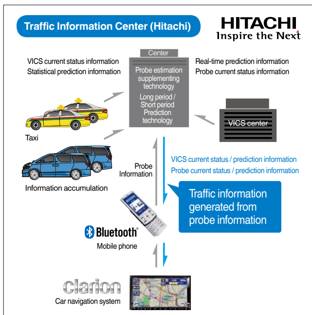
“Online Traffic Information Search” Uses Real Time Information for a High Degree of Traffic Congestion Avoidance
