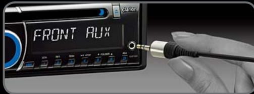
Front AUX Input for connection of portable audio player or other equipment.
