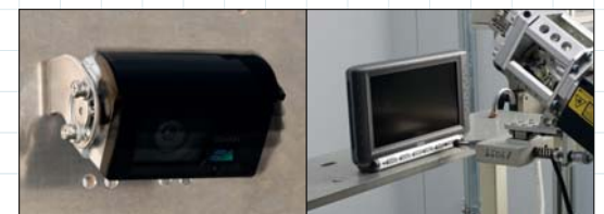
Repetition durability test (to check camera's shutter release and monitor's controls)
