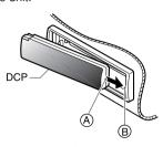
2. Press the left side © of the DCP carefully to fit it in place.
