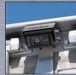
CCD camera mounted on vehicle.
