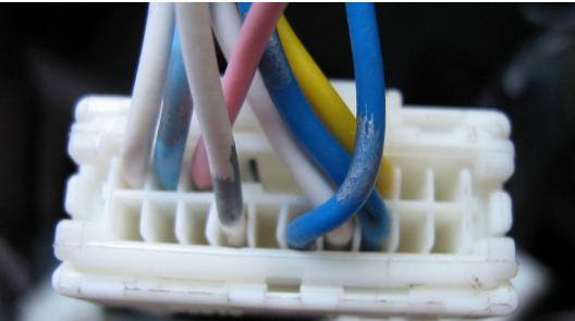
**BLACK to Pin No. 24 vehicle wire colour Blue/Grey rings in 16 way connector.**
