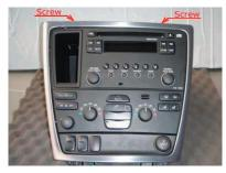
Remove the two torx screws. Remove the plastic trim by using a plastic wedge.
