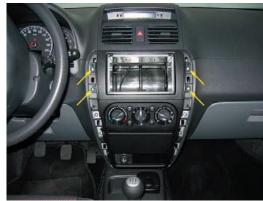
Place the replacement panel. Place the metal 2-DIN bracket
