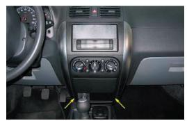
Remove plastic trim around radio & heating panel. Use plastic wedge and start at the location of the arrows.
