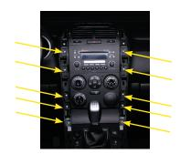
Remove the original radio bracket and fan control panel. This is tighten with screws at the location of the arrows.
