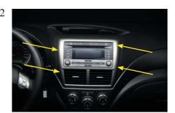
Remove the panel around the radio at the location of the arrows. Use a plastic wedge.
