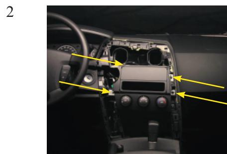
Remove the original bracket. This is tighten by four screws at the location of the arrows.
