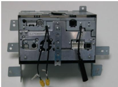
Tighten the headunit onto the metal band. There are various positions of the metal band possible. Choose the positions which gives the best result.
