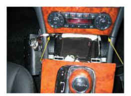
Remove the wooden panel with a torx 20.
