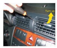
To turn ventilation shaft up, use a screwdriver to unlock the locking clip
