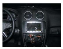
Place replacement panel and the 2- din metal bracket.
