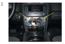
Remove the 2 torx 20 screws at the location of the arrows. Gently pull down the silver bolt.
