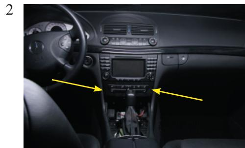
Remove the the screws and remove original storage bin/ CD changer.
