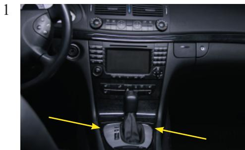
Remove the plastic trim around the gear lever. Remove the ashtray.
