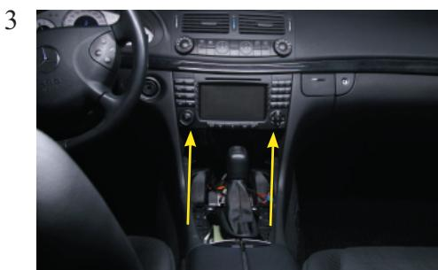
Loosen the screws at the location of the arrows. This is to unlock the original head unit. The screws cannot be removed.
