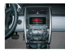
Remove plastic panel around heating instrument with plastic wedge.
