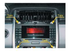
Remove 4x tor x 20 and remove original head unit.
