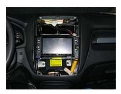
Connect all wiring and place head unit including mounting plates and supporting bracket.
