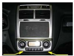
Remove original panel around radio cover and climate control unit. Start at the location of the arrows.
