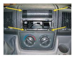
Remove the original bracket using a Philips screwdriver.
