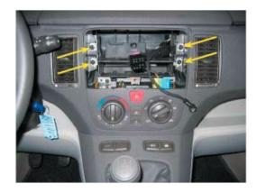
Remove the original bracket. This tighten by four screws witch are marked by the above standing arrows.
