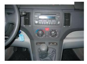
Remove radio using radio removal keys.
