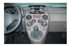
Remove the radio using Philips/ Blaupunkt radio keys.
