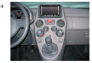
Connect all wiring and place head unit.
