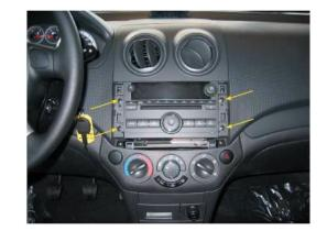
Remove the four screws at the location of the arrows.
