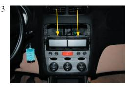
Push the clips at the location of the arrows to remove the cupholder.
