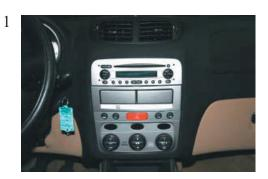
Remove the radio using Philips radio keys.
