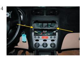
Gently remove the plastic bridge at the location of the arrows using small saw.
