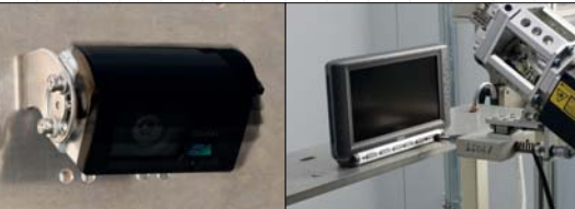
Repetition durability test (to check camera's shutter release and monitor's controls) We check the durability of movable parts such as shutter opening/closing and monitor controls by conducting more than 50,000 operation tests.
