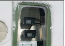
Temperature test Reliability under rapid temperature change is checked, including performance confirmation under high and low temperatures.
