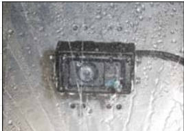
Waterproof test Assuming vehicles are washed by a car wash and exposed to the weather, we check for water penetration inside the camera and determine how watertight the equipment is.
